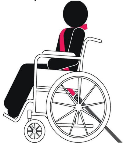
When using as a seat in a vehicle it is extremely important that the passenger follows the diagram (right), ensuring that the harness is fed over the user's shoulder, across the chest and under the side panel of the wheelchair. Ensure the lapbelt is also fed under both side panels.
