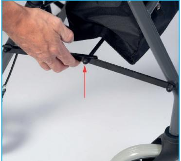
Pull the crossbar handle upwards to unlock the frame, then push the frame together to fold the rollator.
