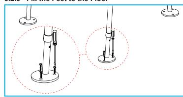
Using an appropriate tool for the chosen fixings, secure the floor fixing feet to the floor.
