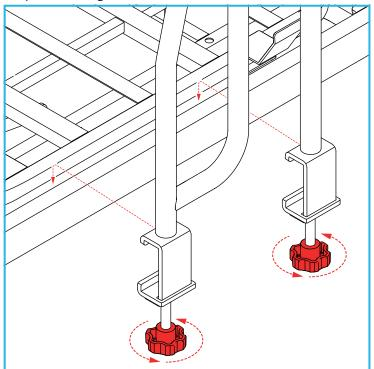
Loosen both hand-wheels fully to enable the fixing bracket to fit over the bed frame.
