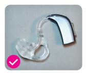
The picture on the left shows the earmould put back the wrong way round. Make sure that the curve of the earmould goes the same way as the curve of your hearing aid, as shown in the picture on the right.
