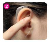
Place the soft tip in your ear with the tail facing backwards (if there is a tail – sometimes the open ear fitting doesn't have one). Push the tip in as far as it will comfortably go, otherwise you won't hear as well as you should.
