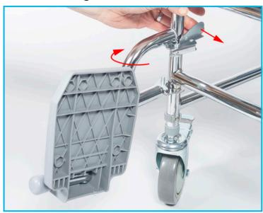
Push the fastener clip to release the footrest.
