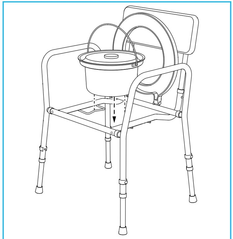
Place the commode pan onto the retainers, on either side of the seat frame.
