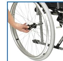
To fit rear wheels depress rubber cover at the centre of the wheel hub and push the wheel spindle firmly into the axle bush, ensuring that both ball bearings are fully exposed beyond the axle bush.
