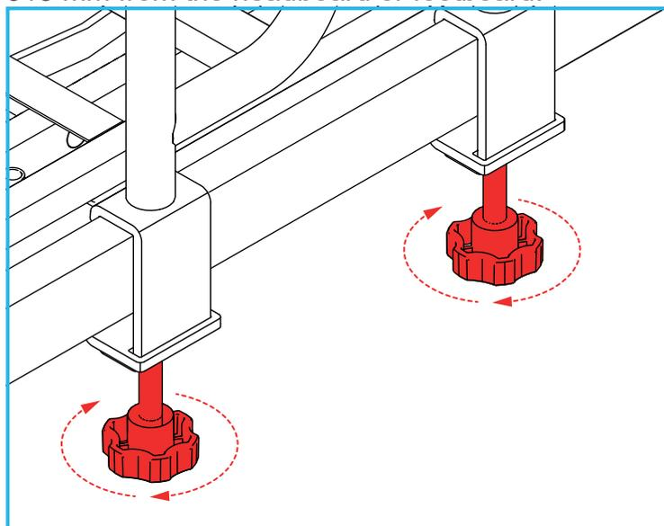
Secure the grab rail to the bed frame by turning both hand-wheels clockwise until the locking brackets are fully tight.
