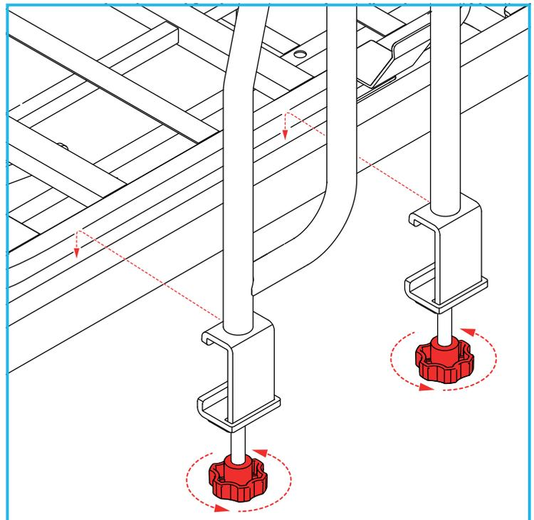
Loosen both hand-wheels fully to enable the fixing bracket to fit over the bed frame.
